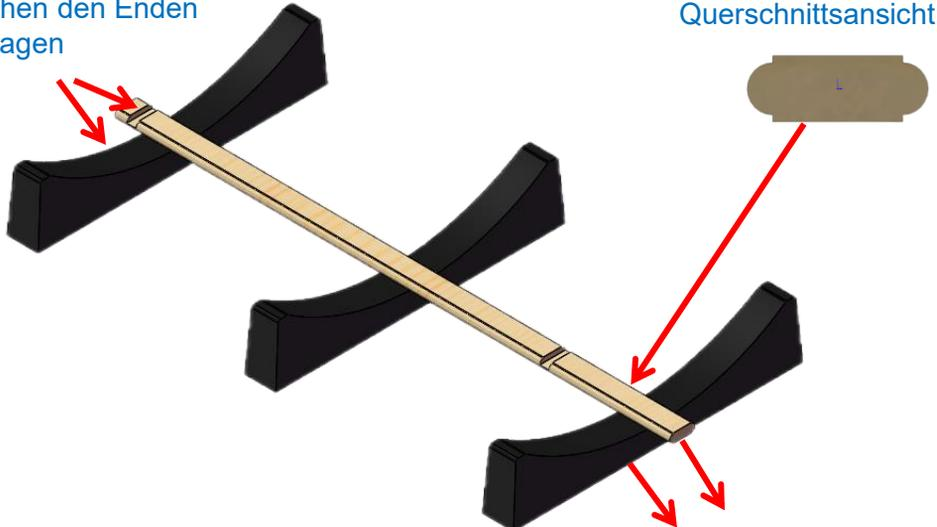
Distance between the ends should be 110mm
